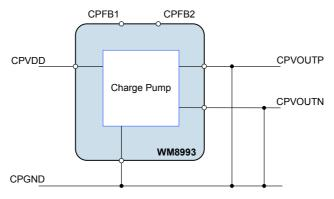
Figure 24 External Configuration when Charge Pump not used
