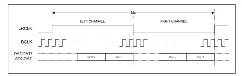
Figure 51 TDM in Right-Justified Mode
