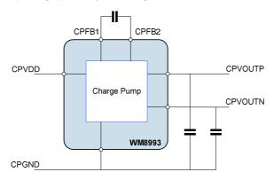
Figure 23 Charge Pump External Connections
