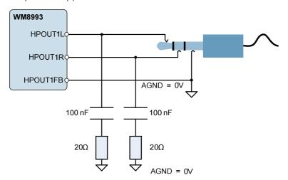
Figure 27 Zobel Network Components for HPOUT1L and HPOUT1R
