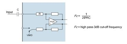
Figure 85 Audio Input Path DC Blocking Capacitor
