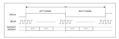
Figure 52 TDM in Left-Justified Mode
