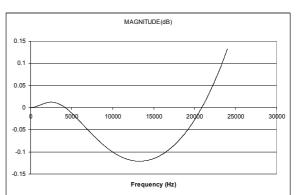
Figure 83 De-Emphasis Digital Filter Response (48kHz)
