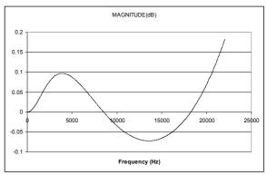
Figure 81 De-Emphasis Digital Filter Response (44.1kHz)
