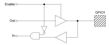
Figure 36 GPIO Pad
