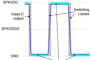
Losses due to resistance between WM8993 and speaker (e.g. inductor ESR) This resistance must be minimised in order to maximise efficiency.
