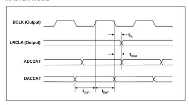
Figure 3 Audio Interface Timing - Master Mode
