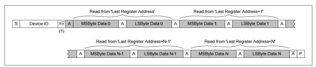
Figure 67 Multiple Register Read from Last Address using Auto-increment
