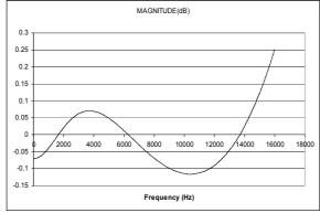
Figure 79 De-Emphasis Digital Filter Response (32kHz)
