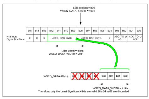
Figure 68 Control Write Sequencer Example
