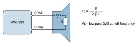
Figure 90 Speaker Equivalent Circuit for Filterless Operation
