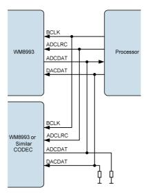
Figure 43 TDM with Processor as Master
