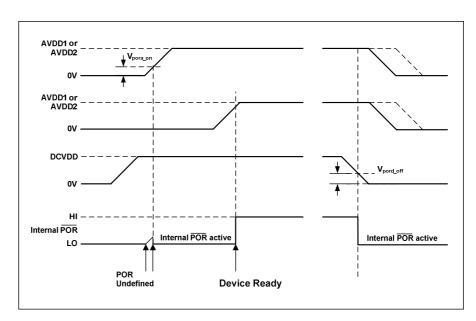
Figure 70 Power On Reset timing - DCVDD enabled first
