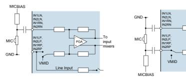
Figure 8 Single-Ended Microphone Input
