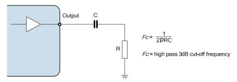
Figure 86 Line Output Path Components
