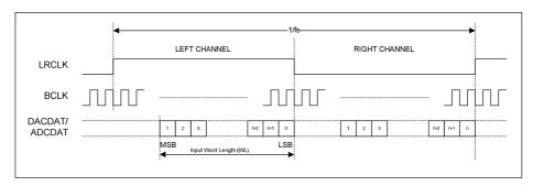
Figure 44 Right Justified Audio Interface (assuming n-bit word length)
