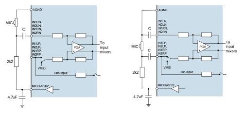
Figure 87 Single-Ended and Differential Microphone Connections
