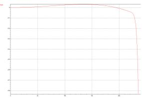
Figure 71 ADC Digital Filter Frequency Response
