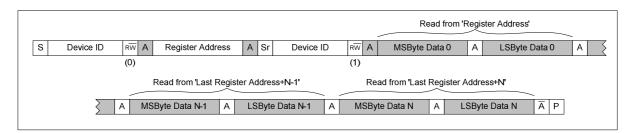
Figure 66 Multiple Register Read from Specified Address using Auto-increment
