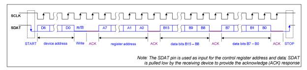
Figure 61 Control Interface Register Write
