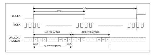
Figure 48 DSP Mode Audio Interface (mode B, AIF\_LRCLK\_INV=1, Master)
