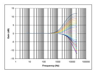
Figure 20 EQ Band 5 – High Freq Shelf Filter Response
