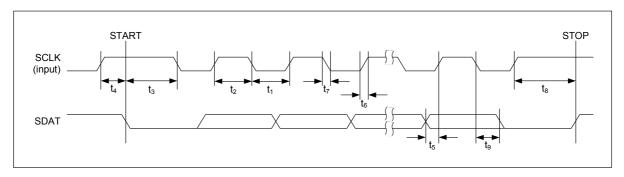
Figure 6 Control Interface Timing
