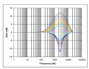
Figure 18 EQ Band 3 - Peak Filter Response
