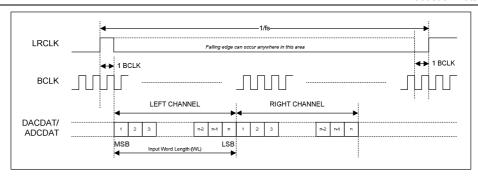
Figure 49 DSP Mode Audio Interface (mode A, AIF\_LRCLK\_INV=0, Slave)
