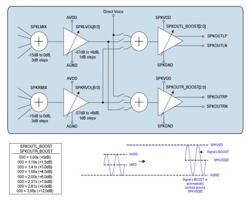
Figure 26 Speaker Output Configuration and AC Boost Operation
