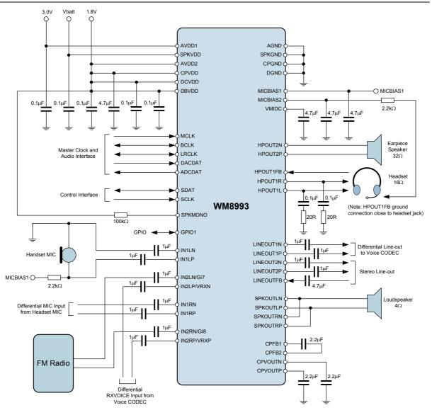
Figure 92 Recommended External Components Diagram – 2W Mono Mode
