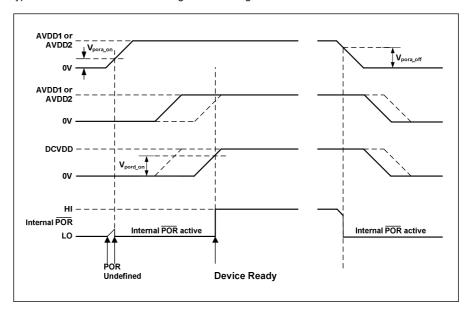
Figure 69 Power On Reset timing - AVDD1/2 enabled first
