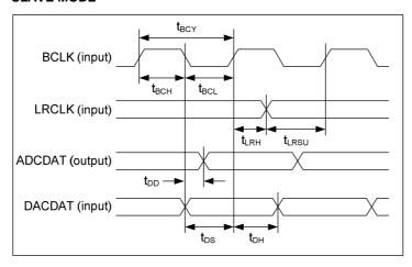
Figure 4 Audio Interface Timing - Slave Mode
