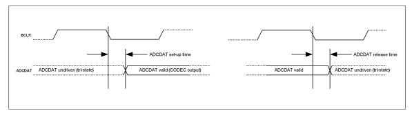
Figure 5 Audio Interface Timing - TDM Mode
