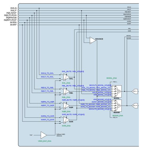
Figure 7 Control Registers for Input Signal Path
