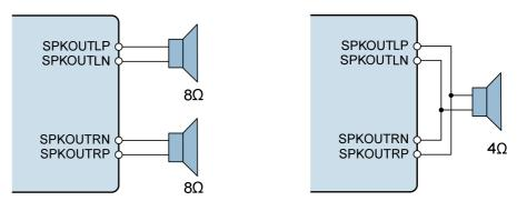
Figure 25 Mono and Stereo Speaker Output Configuration
