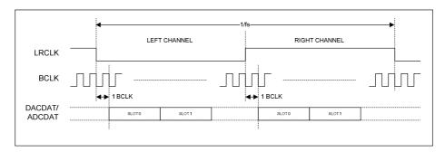
Figure 53 TDM in I<sup>2</sup>S Mode
