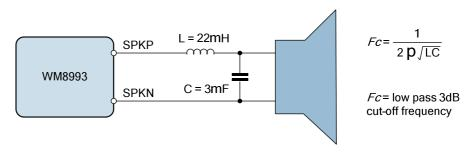
Figure 89 Class D Output Filter Components
