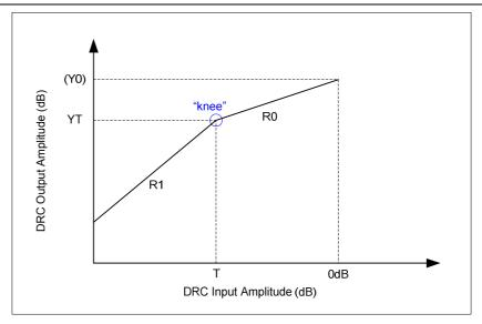
Figure 15 DRC Compression Characteristic
