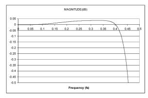
Figure 78 DAC Digital Filter Ripple (Sloping Stopband Mode)
