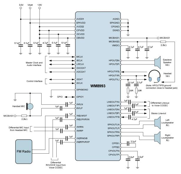
Figure 91 Recommended External Components Diagram - 1W Stereo Mode
