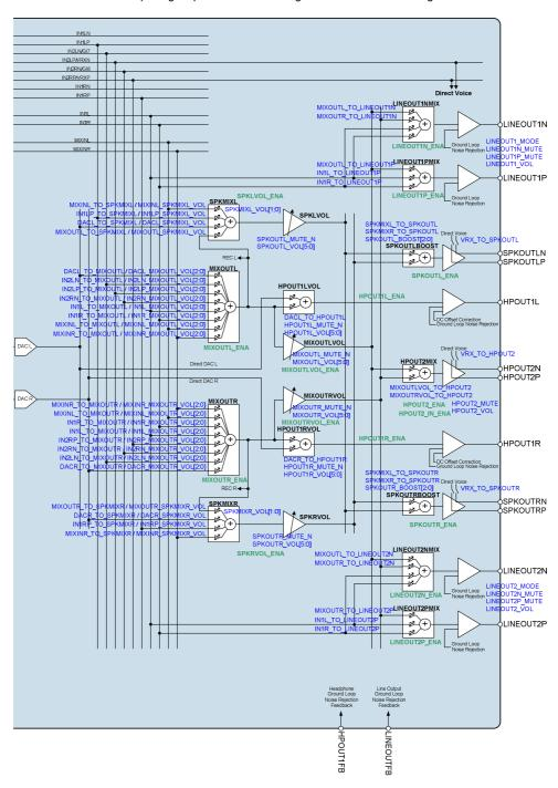
Figure 22 Control Registers for Output Signal Path
