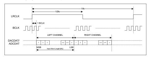
Figure 47 DSP Mode Audio Interface (mode A, AIF\_LRCLK\_INV=0, Master)
