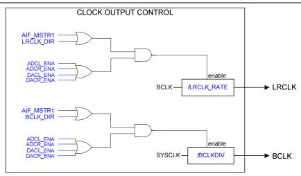
Figure 56 Digital Audio Interface Clock Control
